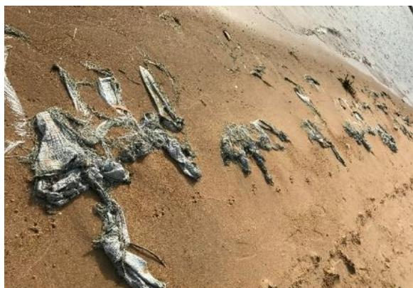
Fig. 6 The Jute Sacks for Erosion Protection Failed (Source: Author's Photograph)
